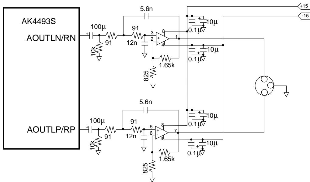
Figure 81. External LPF Circuit Example 3 (fc = 178 kHz(typ), Q = 0.67(typ))
