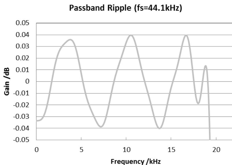
Figure 12. Low Dispersion Short Delay Filter Passband Ripple
