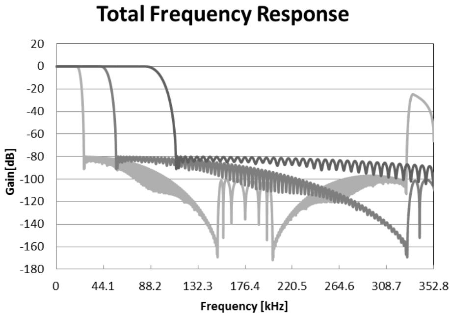
Figure 11. Low Dispersion Short Delay Filter Frequency Response
