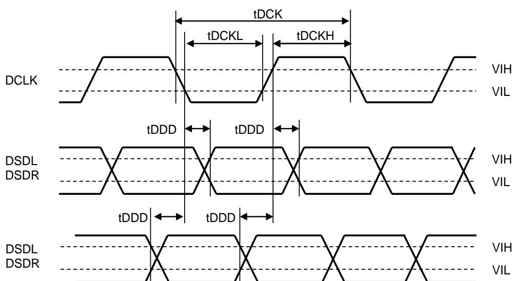
Figure 17. Audio Interface Timing (DSD Phase Modulation Mode, DCKB bit = "0")
