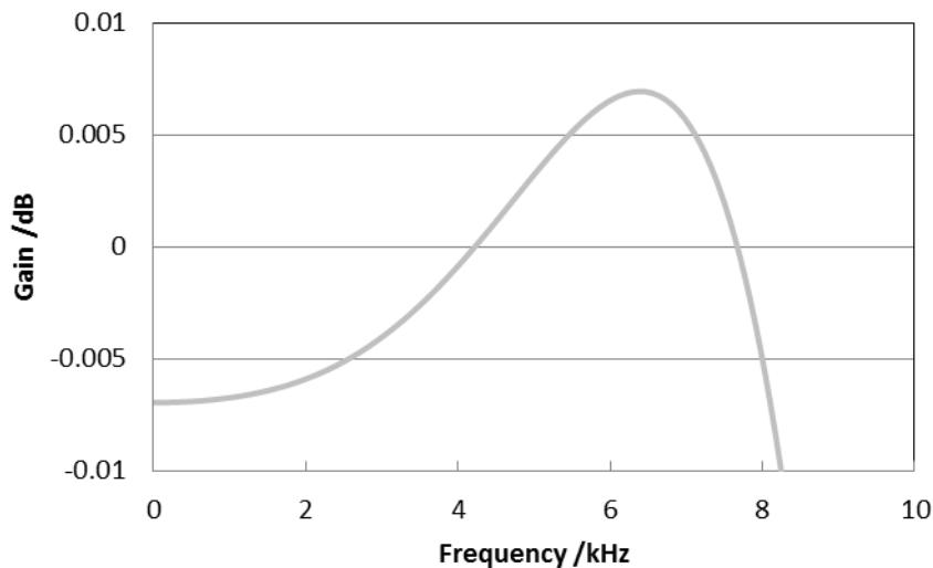
Figure 6. Slow Roll-off Filter Passband Ripple
