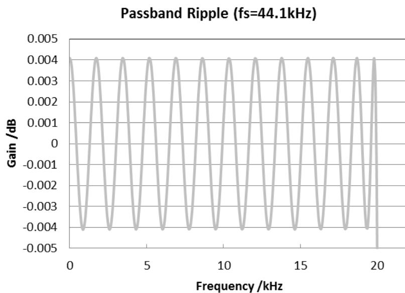
Figure 8. Short Delay Sharp Roll-off Filter Passband Ripple
