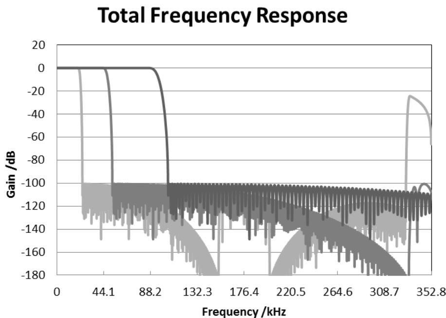
Figure 7. Short Delay Sharp Roll-off Filter Frequency Response
