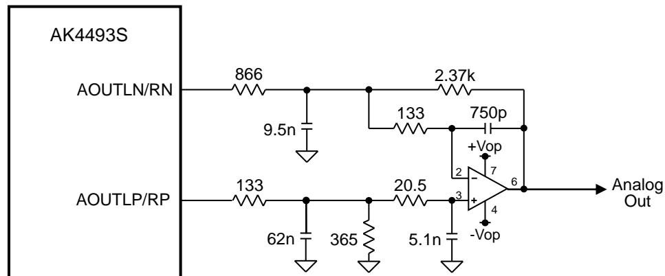
Figure 79. External LPF Circuit Example 1 (fc = 104 kHz(typ), Q = 0.690(typ))
