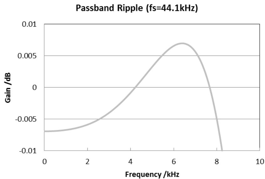
Figure 10. Short Delay Slow Roll-off Filter Passband Ripple
