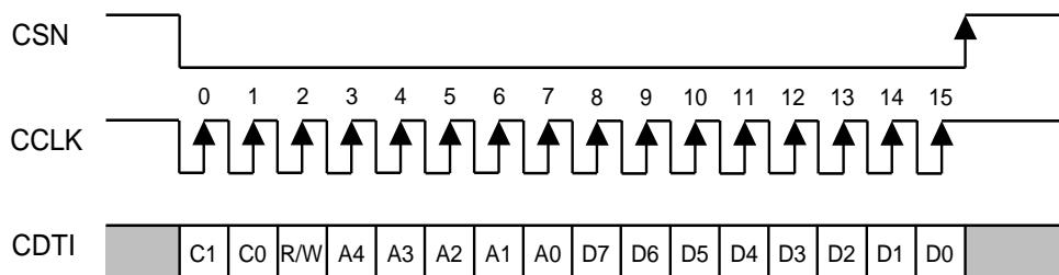
C1-C0: Chip Address (C1 bit = CAD1 pin, C0 bit = CAD0 pin)
