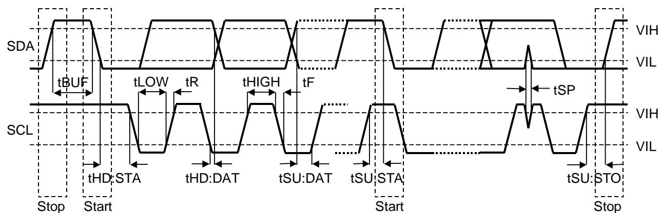
Figure 20. I<sup>2</sup>C Bus mode Timing
