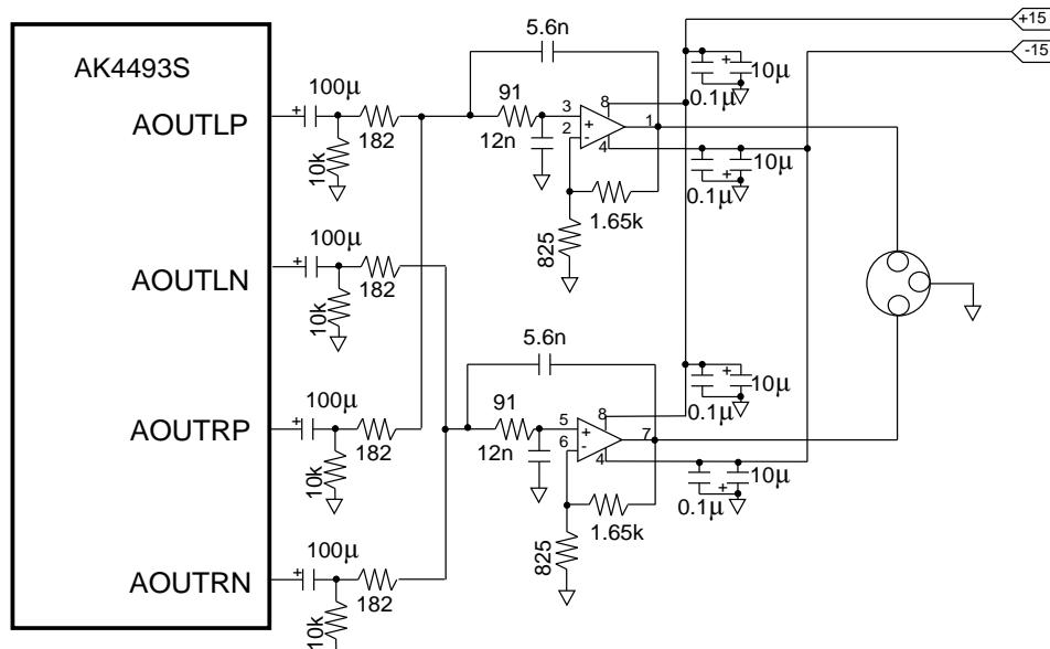
Figure 82. External LPF Circuit Example for Mono mode (fc = 178 kHz(typ), Q = 0.67(typ))
