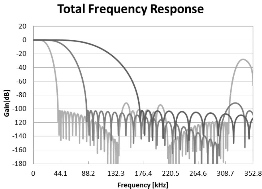
Figure 9. Short Delay Slow Roll-off Filter Frequency Response
