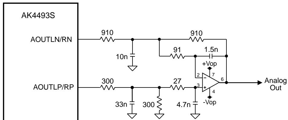
Figure 80. External LPF Circuit Example 2 (fc = 133 kHz(typ), Q = 0.677(Typ))
