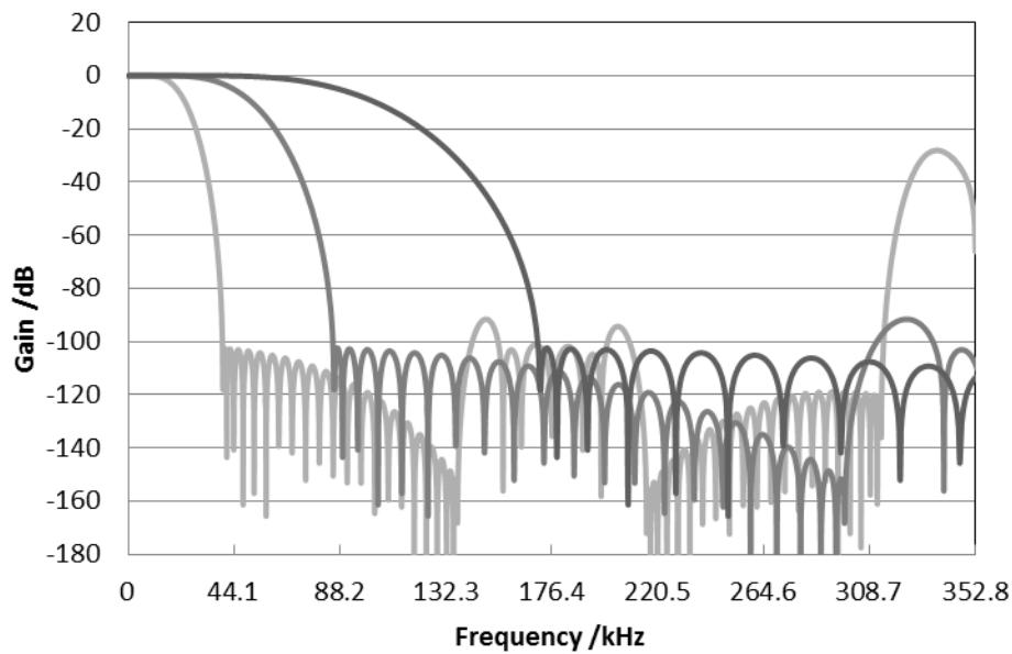
Figure 5. Slow Roll-off Filter Frequency Response
