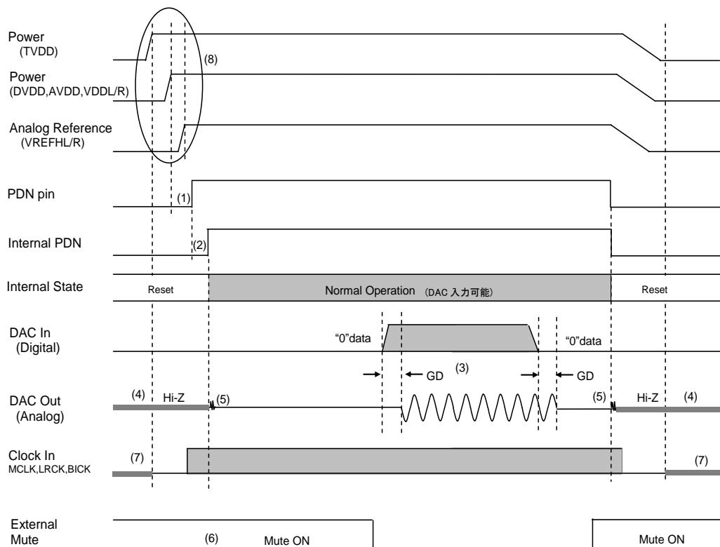
Figure 59. Power-up/down Sequence Example (Pin Control Mode, LDOE pin = “L”)
